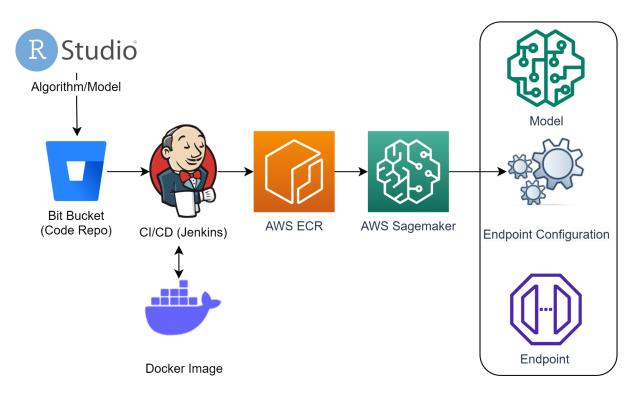
The custom Algorithm/Model is created using RStudio on our machine which has a satisfactory result we name it (Train.r) which is the ENTRYPOINT in our case and has both train and serve function declared in it, the serve function uses Plumber library as it provides simple and quick api functionality and we have a Dockerfile for configuring our container
